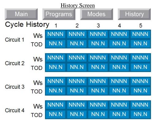
The **History** screen is accessed by touching the button at the top of the Main screen. This screen is always available and does not require a login. This screen shows the history of the last 5 solder cycles of each circuit for troubleshooting purposes. The total energy in WS and the Time of Delivery(TOD) to deliver that energy.
