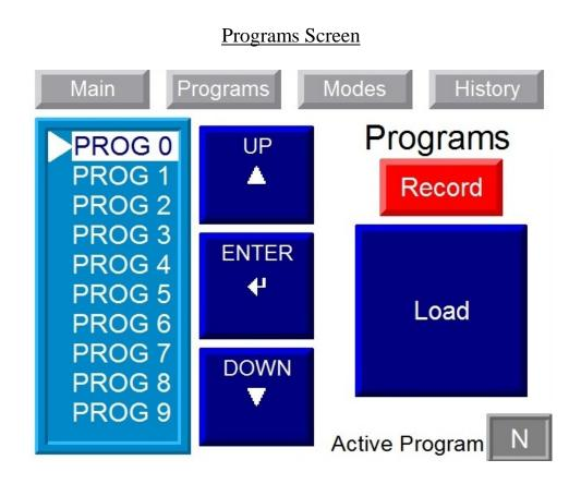
The **Programs** screen is accessed by touching the button at the top of the Main screen. This screen is available only when logged in to the controller. This is used to save and recall programs for use with different solder tools or for different products. There are 10 programs available numbered 0-9. The program number in use is displayed in the "Active Program" box.
