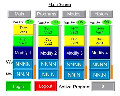
The **MAIN** Screen is used to monitor soldering operation and access other parameters for soldering.
