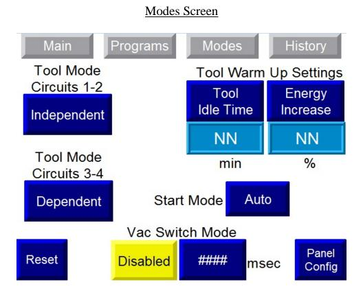
The **Modes** screen is accessed by touching the button at the top of the Main screen. This screen is available only when logged in to the controller. This is used to set operating modes in the Q-box.
