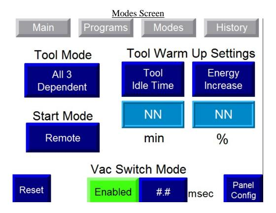
The **Modes** screen is accessed by touching the button at the top of the Main screen. This screen is available only when logged in to the controller. This is used to set operating modes in the Q-box.
