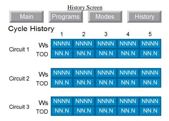
The **History** screen is accessed by touching the button at the top of the Main screen. This screen is always available and does not require a login. This screen shows the history of the last 5 solder cycles of each circuit for troubleshooting purposes. The total energy in WS and the Time of Delivery(TOD) to deliver that energy.
