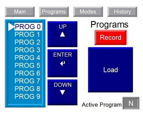
The **Programs** screen is accessed by touching the button at the top of the Main screen. This screen is available only when logged in to the controller. This is used to save and recall programs for use with different solder tools or for different products. There are 10 programs available numbered 0-9. The program number in use is displayed in the "Active Program" box.
